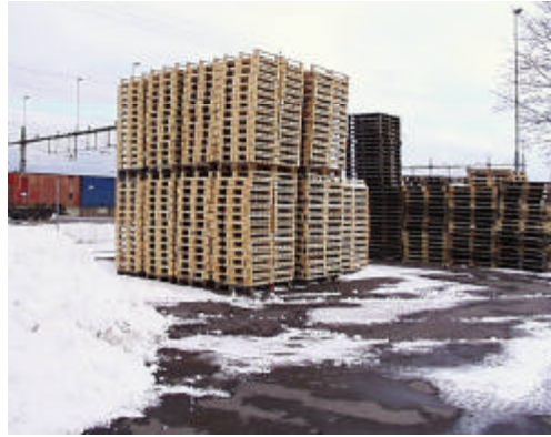
Picture 4 Don't store pallets outdoors. Don't stack pallets directly upon each other - put sticks (skids) between the unit loads
